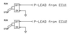
When P-lead input is grounded, ignition operation will STDP When P-lead input is open, ignition operation will RUN
