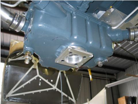
Attach the sump adapter to your engine sump using the included 5/16"-24 x 1 1/4" socket head screws. Use Ultra Black Silicone Gasket Maker between the engine sump and the sump adapter. Use blue loctite on the 5/16" allen head screws and torque to approx 180 in. lbs.
