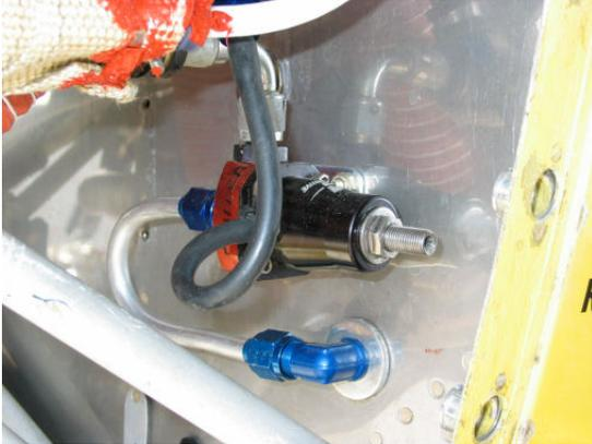
The Fuel Pressure Regulator is typically mounted to the firewall and fed from the fuel line leaving the fuel injectors. The side port is the INLET to the regulator. The bottom port is the OUTLET from the regulator that will then return to the header tank or fuel selector return plumbing.
